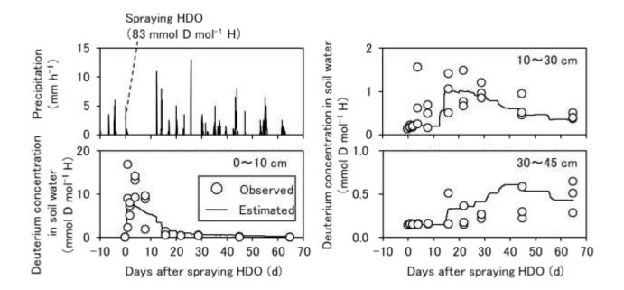
Fig. 1 Observed and estimated concentrations of deuterium in soil water of the 1-yr meadow where deuterium-enriched water (HDO) was sprayed to the soil surface. Replicated data are separately presented for each soil layer.
