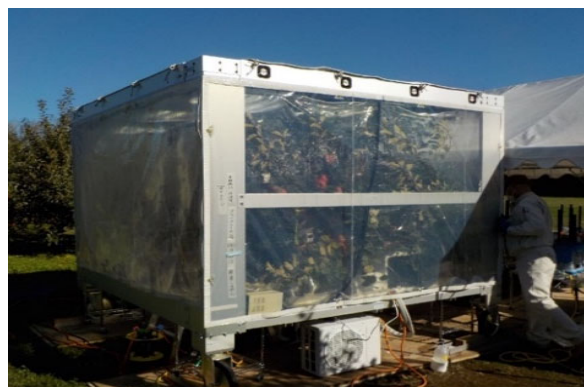
Fig. 1 A photo during the ^{13}\text{CO}_2 exposure experiment using a mature apple tree in an orchard.
